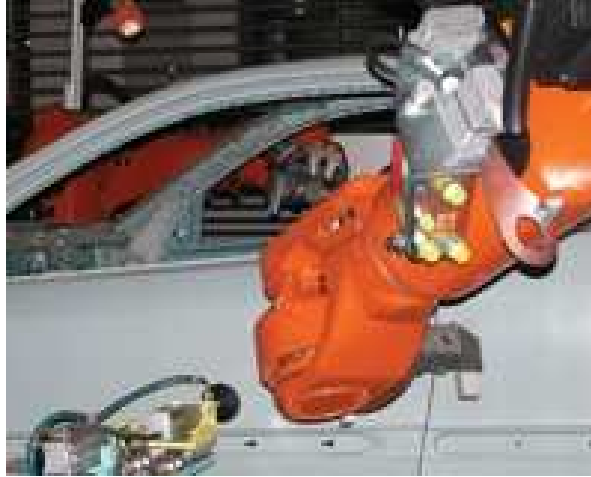
Graph 37 – INOS - Gap & Flush Installation
